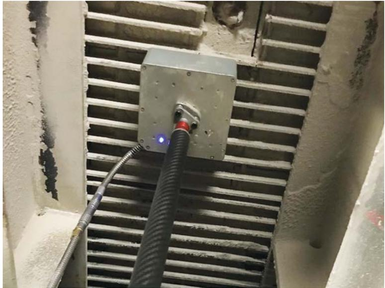
SmartMelter sensor to map metal infiltration in a furnace bottom.
